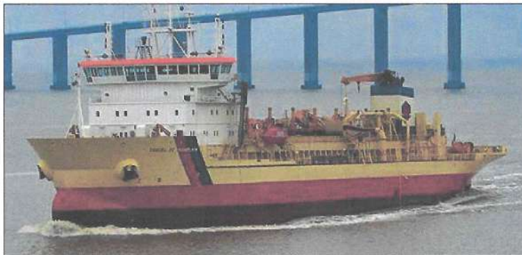
DP's Samuel de Champlain - an 8,500 m 3 Trailing Suction Hopper ( TH ) Dredge
